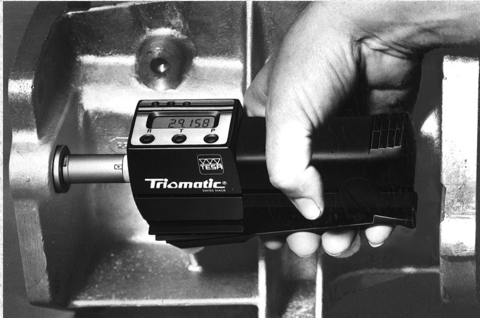
Figure 35.7 An electronic gage for measuring bore diameters. The measuring head is equipped with three carbide-tipped steel pins for wear resistance. The LED display reads 29.158 mm. Courtesy of TESA SA.
