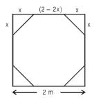
Let the length of the edge cut at each corner be x m. Since the resulting figure is a regular octagon,
