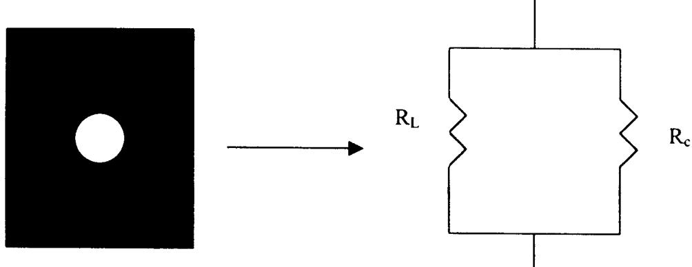
For the lead,  $R_L = \frac{l}{\sigma_L S_L}, \quad S_L = d^2 - \pi r^2 = 9 - \frac{\pi}{4} \text{ cm}^2$
