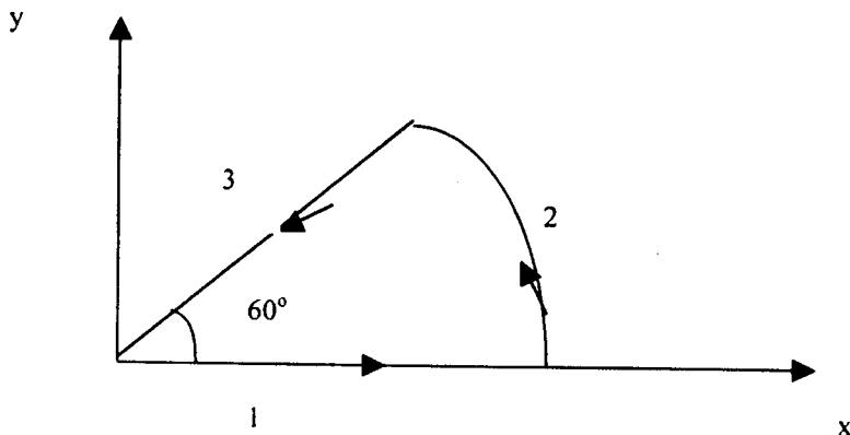
$$\oint_L \bar{A} \bullet d\bar{l} = (\int_1 + \int_2 + \int_3) \bar{A} \bullet d\bar{l} = C_1 + C_2 + C_3$$
