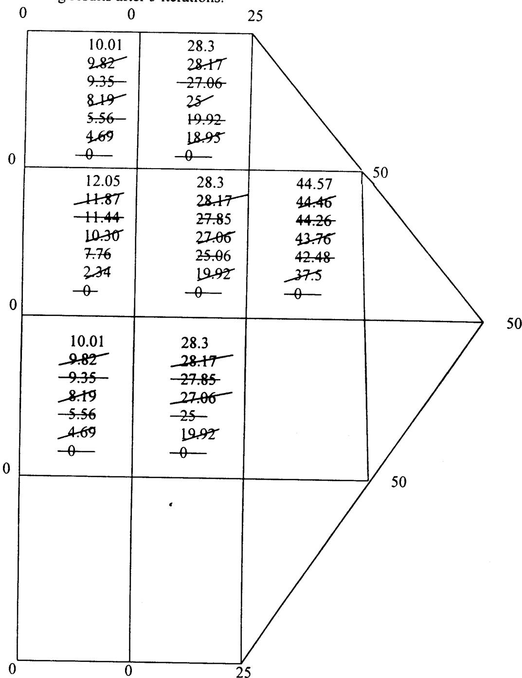
**P. E. 15.4** (a) Using the program in Fig. 15.16 with  $NX = 4$  and  $NY = 8$ , we obtain the potential at center as
