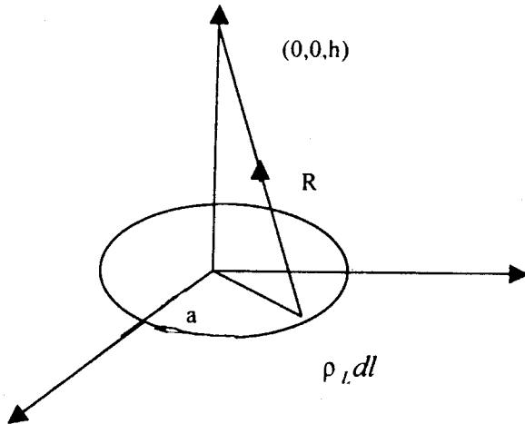
$$\bar{D} = \int \frac{\rho_L dl \bar{R}}{4\pi R^3}, \quad \bar{R} = -a\bar{a}_\rho + h\bar{a}_z$$
