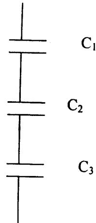
$$\frac{l}{C} = \frac{l}{C_1} + \frac{l}{C_2} + \frac{l}{C_3}$$
