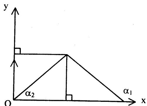
$$\bar{H}_3 = \frac{10}{4\pi\sqrt{20}} \left( -\frac{8}{\sqrt{84}} - 0 \right) \bar{a}_x \times \left( \frac{2\bar{a}_x - 8\bar{a}_y}{\sqrt{20}} \right) = \frac{\bar{a}_y + 2\bar{a}_z}{\pi\sqrt{21}}$$
