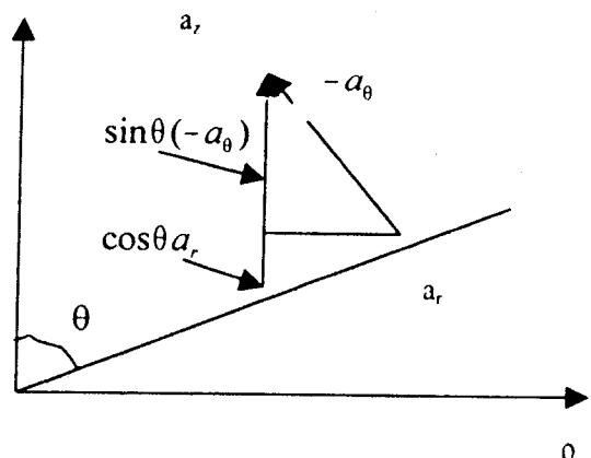
$$\begin{bmatrix} \bar{a}_\rho \\ \bar{a}_\phi \\ \bar{a}_z \end{bmatrix} = \begin{bmatrix} \sin \theta & \cos \theta & 0 \\ 0 & 0 & 1 \\ \cos \theta & -\sin \theta & 0 \end{bmatrix} \begin{bmatrix} \bar{a}_r \\ \bar{a}_\theta \\ \bar{a}_z \end{bmatrix}$$
