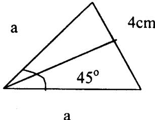
$$a \sin \frac{45^\circ}{2} = 2 \quad \longrightarrow \quad a = \frac{2}{\sin 22.5^\circ} = 5.226 \text{ mm}$$
